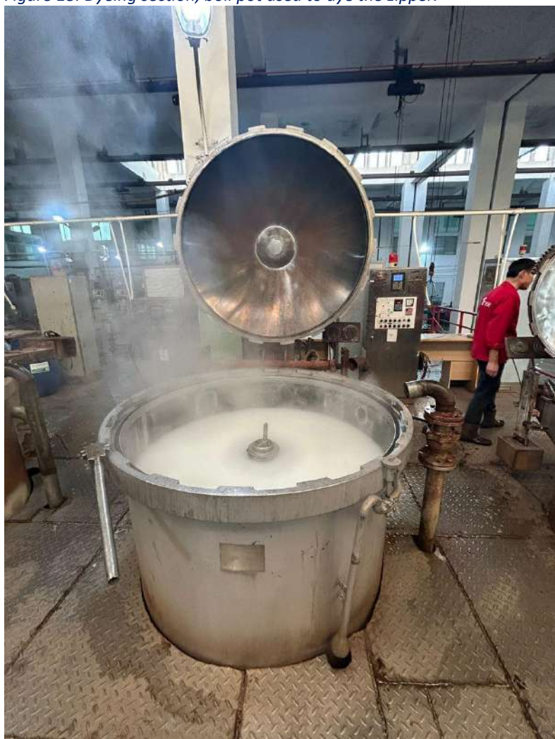
Figure 18: Dyeing section, boil pot used to dye the zipper.
