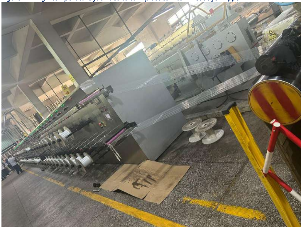
Figure 14: High-temperature facilities to turn plastics into Threads for zipper
